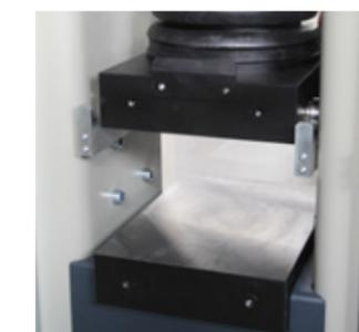
Sliding of the block upper platen on the solid rail system
