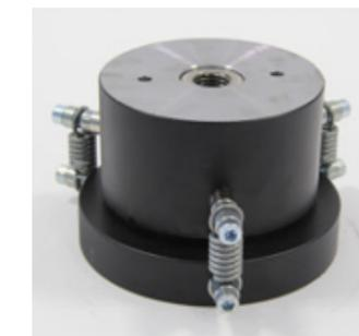
Upper platen and spherical seat strictly conforming to ASTM C39, AASHTO T22
