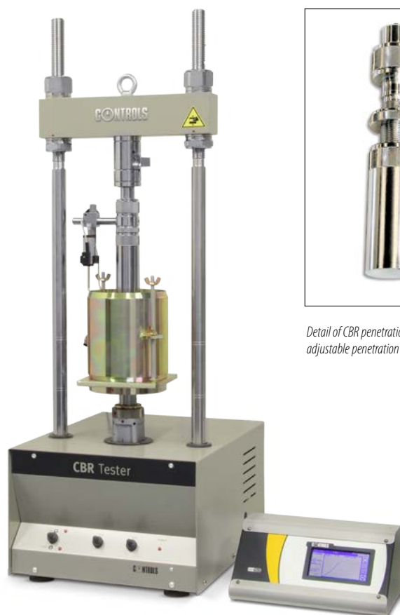
CBR loading press equipped with CBR mould and digital data acquisition system (DIGIMAX TOUCH acquisition unit)
