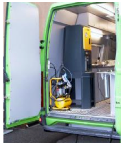
Gyrocomp installed inside a van as a road mobile laboratory
