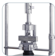
Flexural test on mortar prisms 40 x 40 x 160 mm
