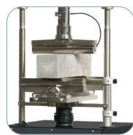
Flexural tests on concrete beams, concrete and clay tiles
