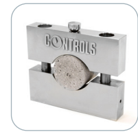
Splitting tensile test of intact core specimens
